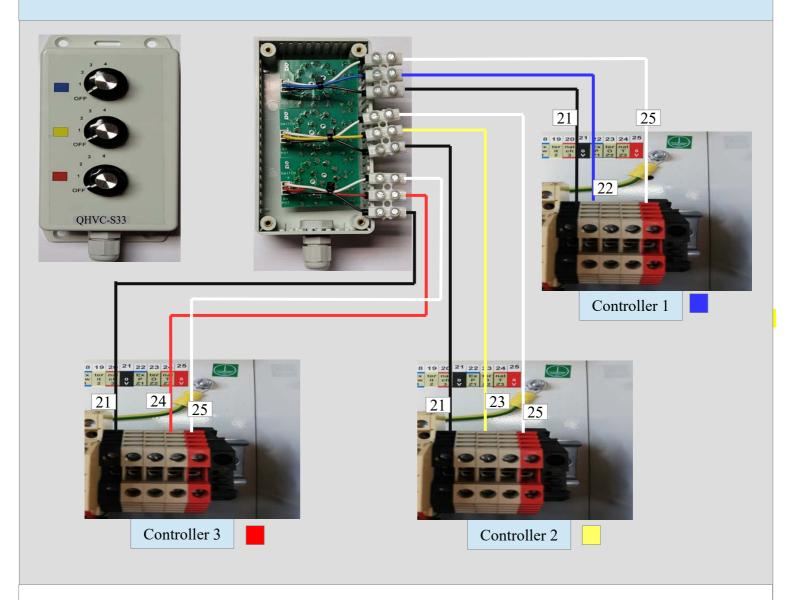
When using a QHVC-S33 to control 3 Seperate QHC18M Controllers
